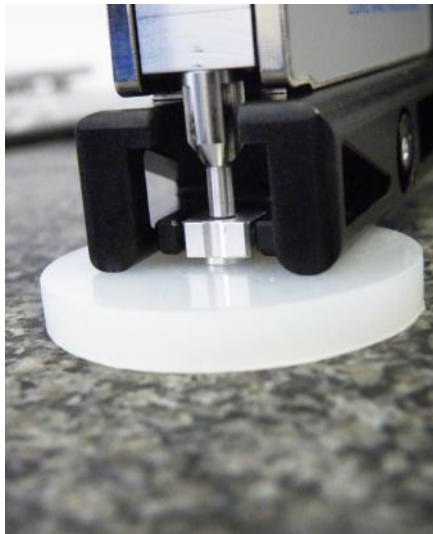
Measurement of IRHD and VLRH with ring adapter on the stand at standard test
